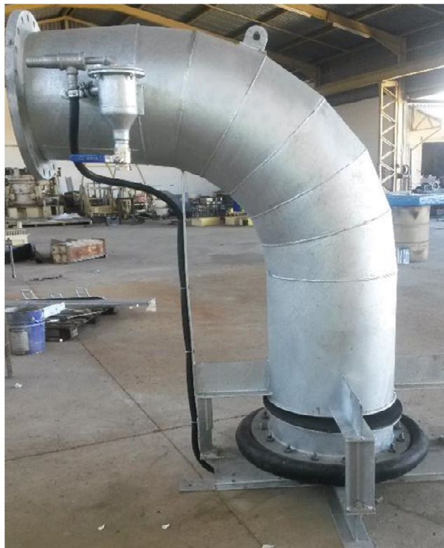
Figure 7. Typical DV to control outflow to bio-filter pond
